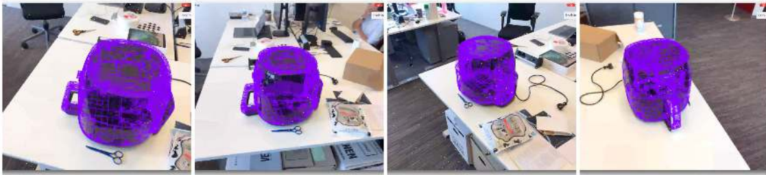
Figure 9.2: Practical Prototype - Augmenting the real airfryer object with an overlay of its 3D CAD model.
